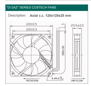
Black fibreglass reinforced plastic (PBT) UL Casing material:
