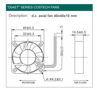
Casing material: Black fibreglass reinforced plastic (PBT) UL
