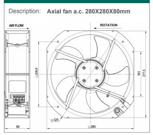
Impeller material: Casing material: Fixing system: Motor protection: Rated temperature range: Electrical connection: Working class of capacitor: Category: Weight: Approvals: black painted metal blades aluminium alloy die casting UNI5076 no 4 holes Ø5.4 thermally protected from -25°C to +70°C by terminal block 3 pins (L-N-PE) class A capacitor run external rotor 2,8 kg CE
